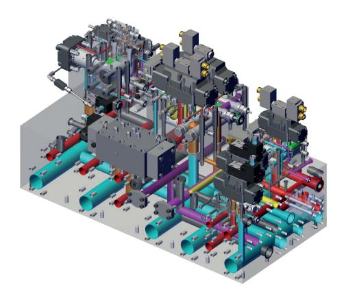
Starting from customer specifications, Flodraulic Industrial designs and manufactures integrated manifolds. Prior to delivery each manifold is fully tested and certified to guarantee high performance and 100% safety for the operators.
